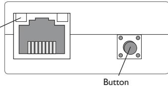
→ In order to connect the KM2 Communication module to the router via WPS, keep the button pressed for 5 s.
