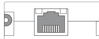
The LAN connector is located on the front side of the device and supports transfer rates of up to 100 MBit per second.
